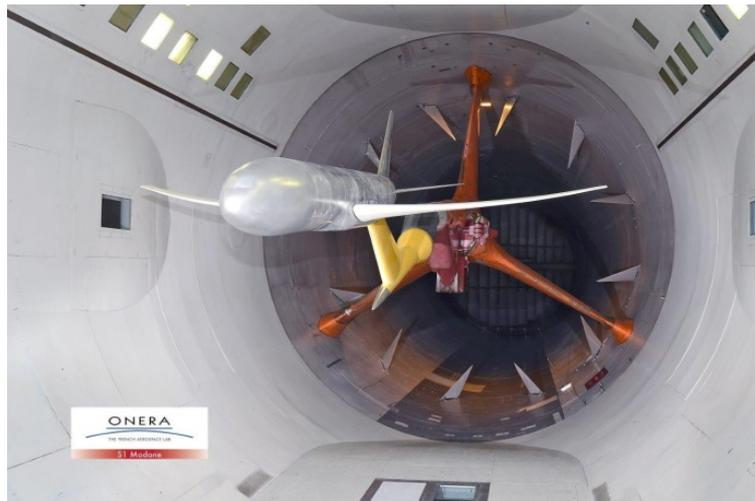
Figure 4: The LRM model in S1MA wind tunnel.
